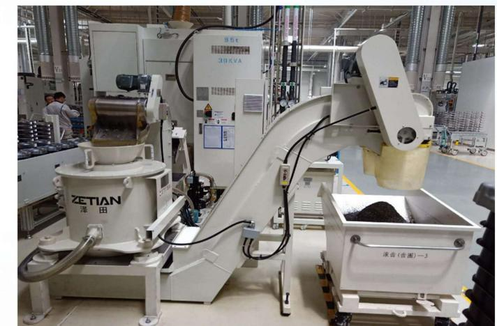
破碎処理装置 Chip Crushing Equipment
