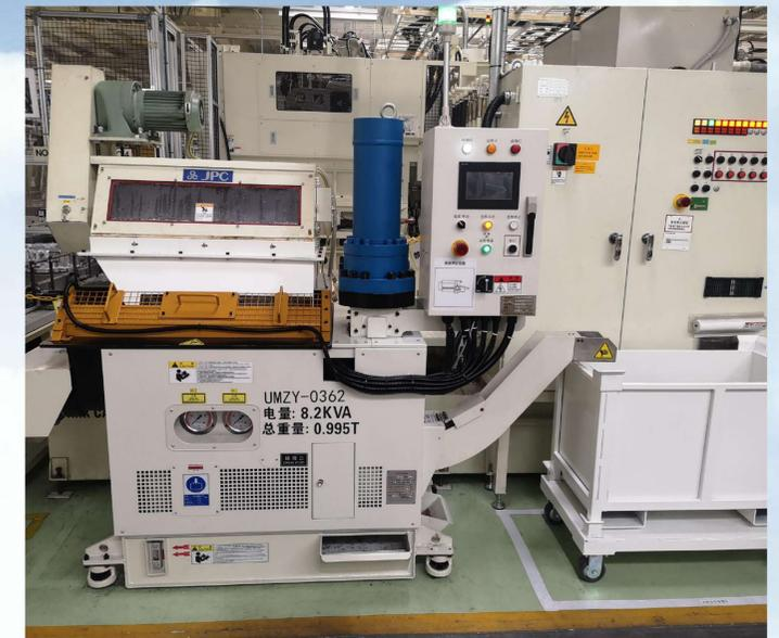
脱油装置 Degreasing Equipment
