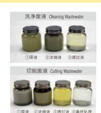
1)Original Waste Liquid 2 Concentrated Liquid 4Finally-treated Liquid ③Permeated Liquid
