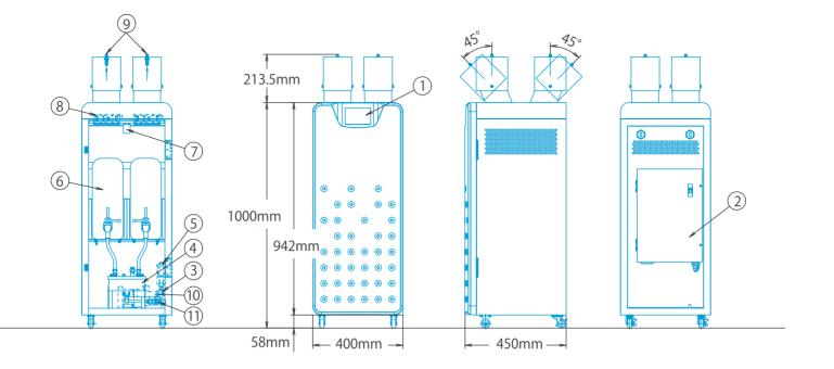
①Operation Panel ②Control Method ③High Pressure Pump ④Storage Tank ⑤Pressure Release Solenoid Valve ⑥Water Tank ⑦Humidity Sensor ⑧Blowing Fan (DC24V) ⑨Spray Nozzle (1.5L/L) ⑩Water Supply Side Air Bleeding/ Storage Tank Drain Valve ⑪Drain (Outer Diameter φ10 Tube Connection)
